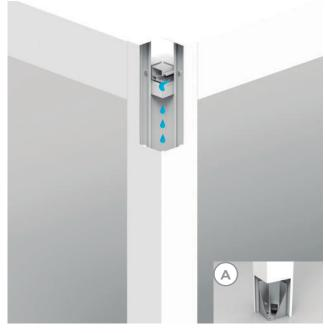
EXAMPLE FREE DRAINAGE SYSTEM & PILLAR BOTTOM SUPPORT (Figure A)
